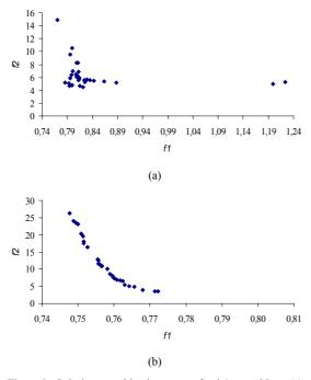
Figure 5 - Solutions on objective space of volt/var problem: (a) first generation; (b) last generation (3000) – Approximation of Pareto Set.
